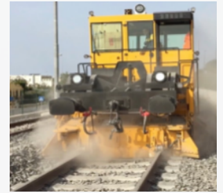
The central ploughs can work both forward and reverse.
